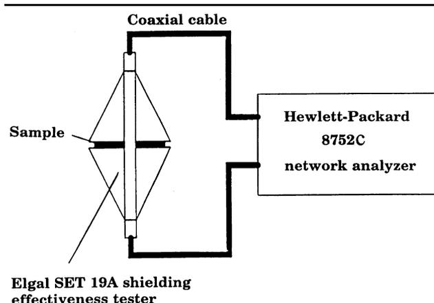
Fig. 1. Set-up for measuring the electromagnetic interference shielding effectiveness.
